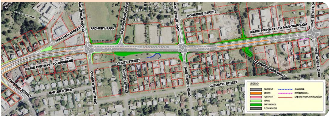
Stage three layout of the Bruce Highway upgrade in Gympie
